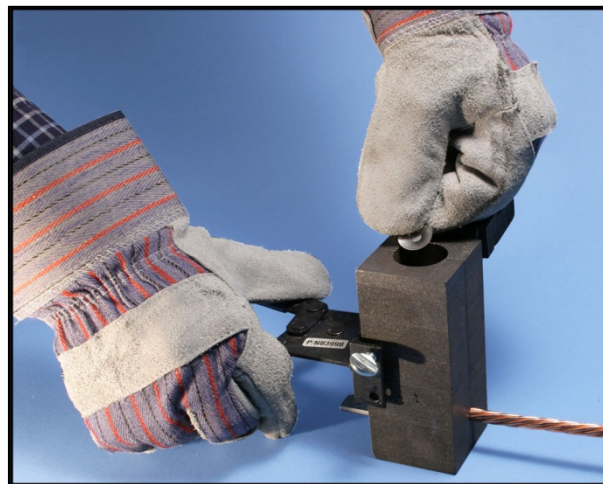
Figure 16. Mold being locked and disk inserted
