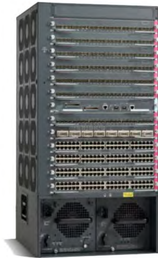
Figure 17-2 Twenty Rack Unit (20 RU) Network Switch Chassis with Installed Switches
